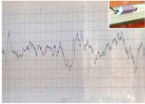
Figure 8: Roughness of the Steel Tool ( R_a = 0.16 \mu\text{m} )
